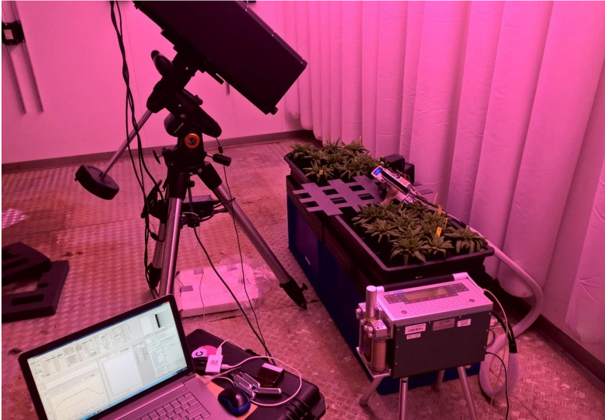
Figure 5 Experimental set-up of combined light-induced fluorescence transient (LIFT) and gas exchange measurements. The leaf was placed in a LI-COR chamber head which allowed measurements of CO 2 assimilation in a highly controlled environment. LIFT device was mounted to an tripod allowing perpendicular fluorescence measurements of Arabidopsis leaves at 60 cm distance. Measurements took place in the dark using the actinic blue light of the LIFT device as light source.
