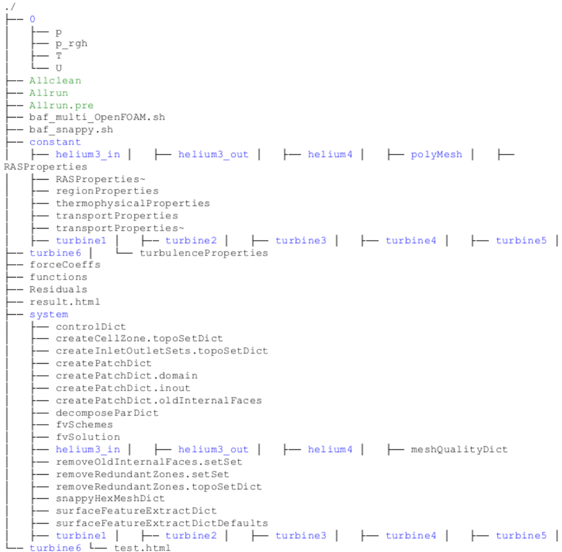
Figure A.1: Example case structure for a CHTMULTIREGIONSIMPLEFOAM case
