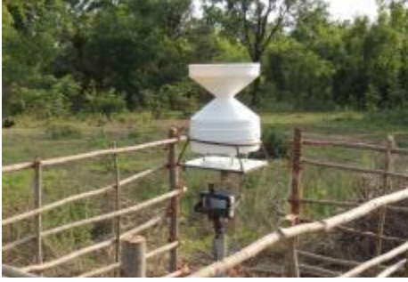
Figure 4.2. Tipping bucket rain gauge installed at Tossahou.
