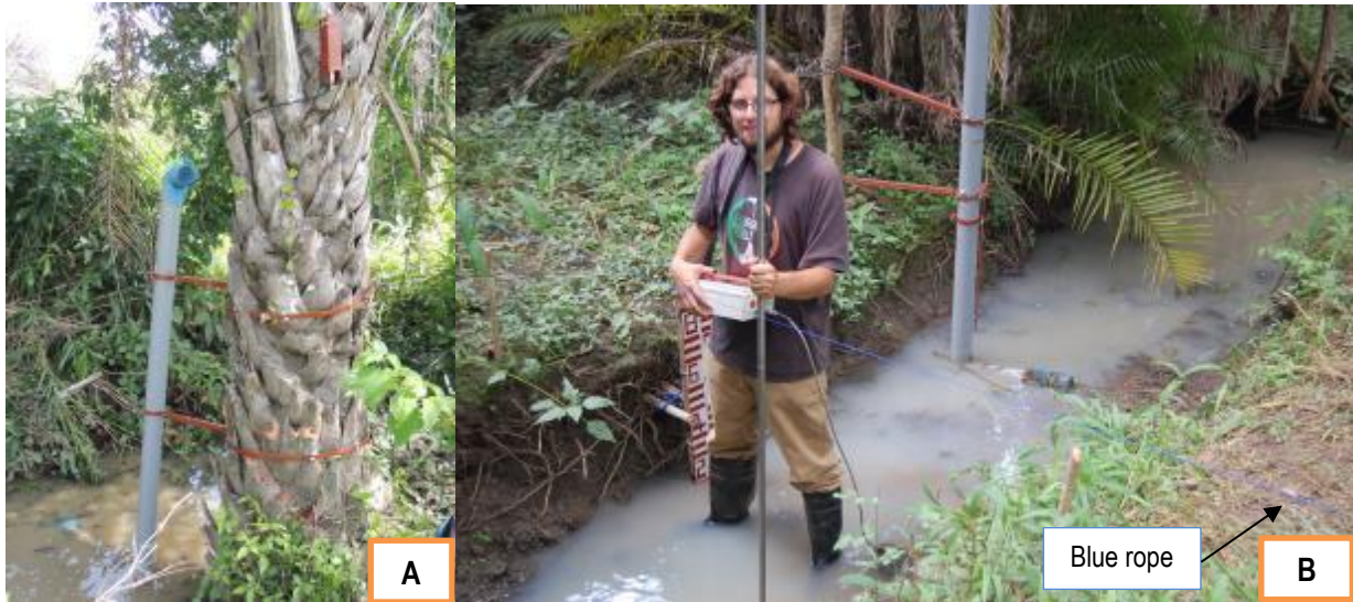
Figure 4.5. (A) Gauging station for recording water level every 5 min at Kounga; and (B) Velocity measurement in Kpandouga at a typical cross-section with the blue rope marking the cross-section (positions of verticals are quite invisible but marked on the rope).
