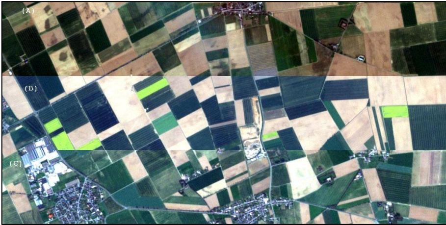
Figure 2.4. Part of the standard L3A RapidEye image from April 02, 2011 (A). The reference image dated April 24, 2011 (B). IR-MAD processed image (C). RGB band combinations are 3-2-1.
