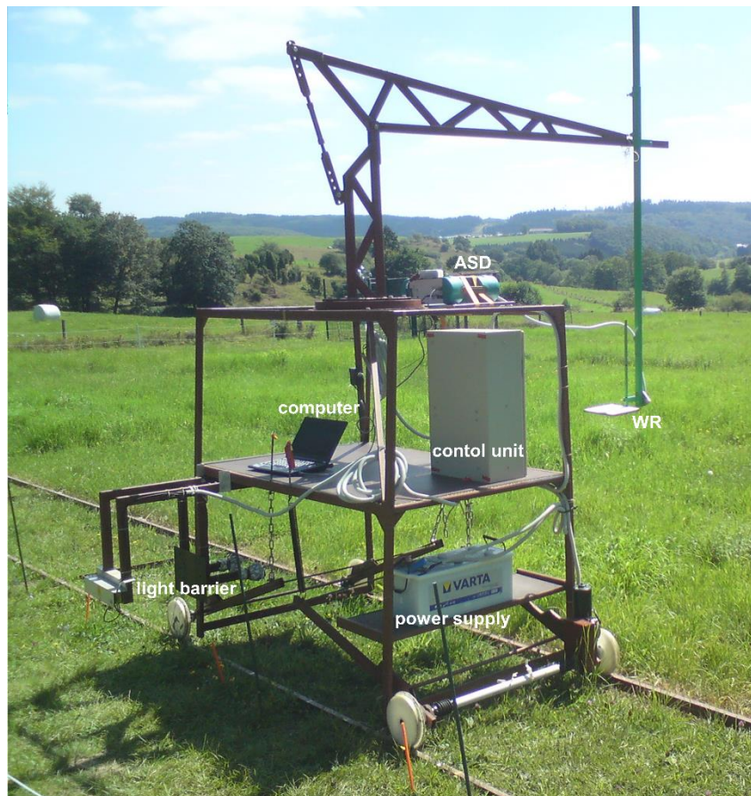
Figure A 1. The crane system installed at the Rengen Grassland Experiment (adapted, Photo: Vittek, M., 2013).
