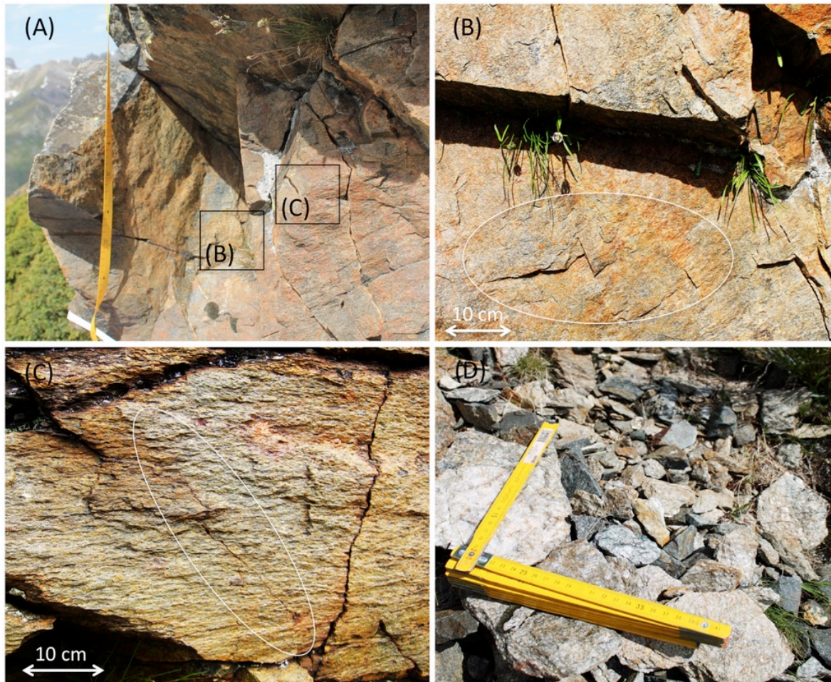
Figure 2.20: A south-exposed, paragneiss rockwall in the Swiss Alps at approx. 2800 m asl (A) with typical fracture patterns (B, C) and detached material at the slope foot (D). In (B) Micro-cracks along pre-existing, slope-parallel foliation and bedding structures and thin flaking of bedrock near-surface could point to thermal stress fatigue. In (C) rectilinear orthogonal micro-cracks independent from schistosity and pre-existing joints could result from thermal shocks.
