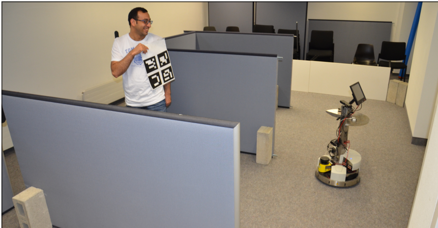
Figure 16: The robot and the user with a board of ArUco markers to simplify pose estimation in the real-world experiment.
