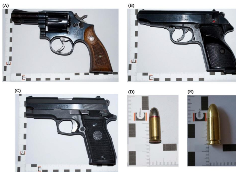
Fig. 1. Overview of used firearms and ammunition for ballistic experiments. (A) a Smith & Wesson revolver caliber 0.38 Special (B) a FÉGARMY Arms Factory semi-automatic pistol caliber 7.65 mm Browning (C) an Astra semi-automatic pistol caliber 9 × 19 mm (D) a semi-jacket soft point bullet (158 gr) fired with revolver caliber 0.38 Special (E) a full metal jacket bullet (124 gr) fired with the two semi-automatic pistols.
