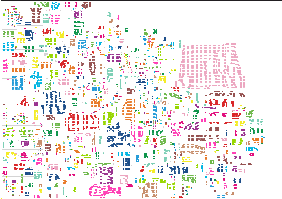
Figure 4.2: The placement with shredded macro fragments on Rosemarie. Fragments colored according to the original macros.
