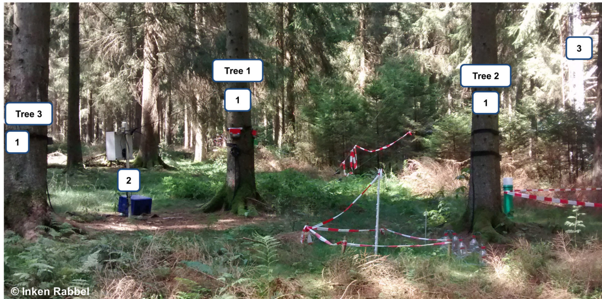
Figure 1.12: Experimental design of a DHC-station: (1) Granier-type sap flow sensors and point dendrometers; (2) Measurements of temperature and relative humidity; (3) Eddy-covariance system belonging to the TERENO project.
