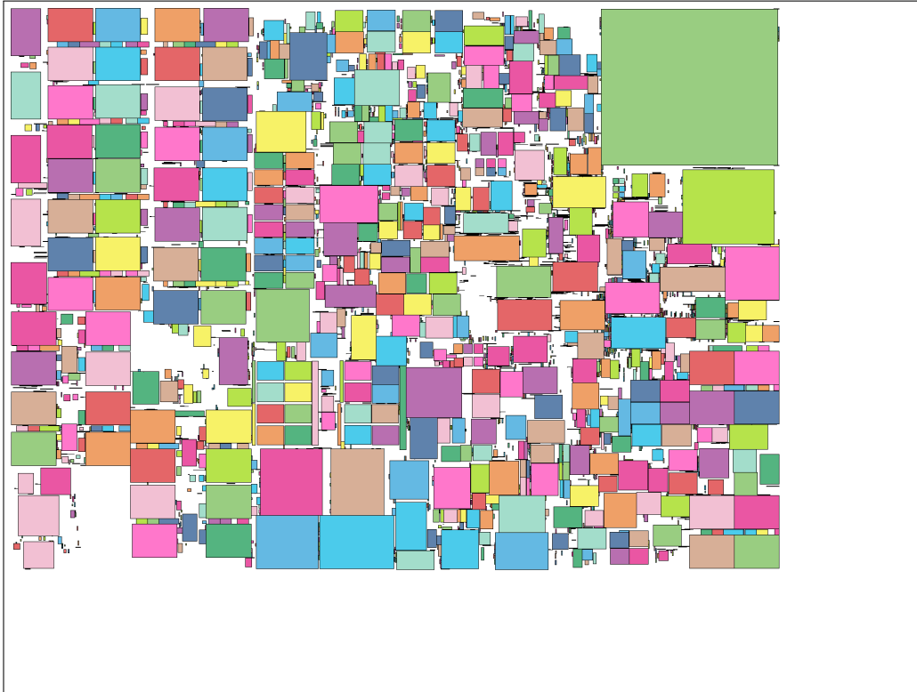
Figure 2.2: Floorplan prototype of a processor core designed with the help of BONNMATCH, reducing area by 30 %. The area shown in this image corresponds to the outline of the original floorplan, the empty white border on the sides is the saved area.
