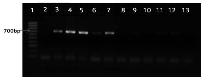
Figure 2.6 1% Agarose gel of A2/J5 ribosomal protein rDNA PCR products. 1: 100bp ladder, 2: Negative control, 3-7: Amplification from infected insect samples, 8-13: weakly amplified samples
