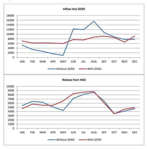
Figure D.2: Flow into and release from HAD without and with GERD
