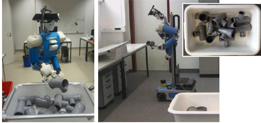
Figure 4.1: Mobile bin picking scenario. Cosero grasps objects from a transport box. It navigates to a processing station and places the objects there.
