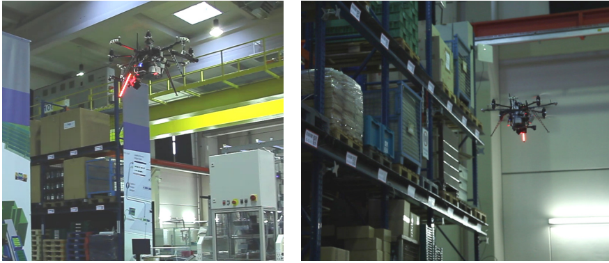
Figure 5.2: Flight in a warehouse. In indoor environments MAVs in general have to operate close to obstacles. Reliable obstacle avoidance is important not only for autonomous, but also for remote-controlled operation in these scenarios.
