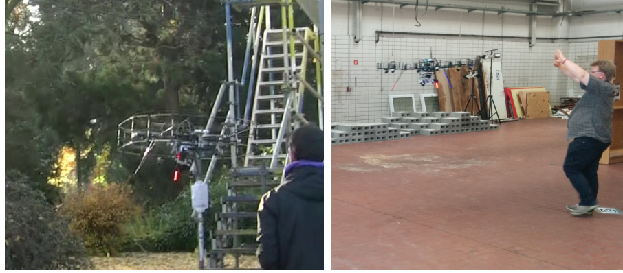
Figure 9.1: Reactive obstacle avoidance. Our local obstacle avoidance algorithm acts as a safety measure between control inputs given by a planning layer or a human pilot remotely controlling the robot. This ensures safe operation in challenging situations. Left: A human pilot manually steers the MAV through a narrow passageway between vegetation and scaffolding leading to a collision that could have been avoided by obstacle avoidance. Right: A person approaches the MAV hover position, the MAV avoids this dynamic obstacle.
