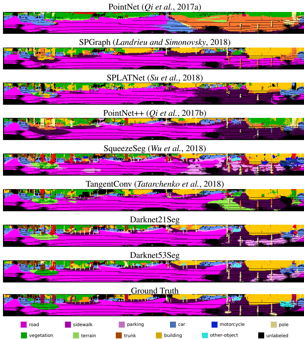
Figure 8.5: Examples of inference for all methods. The point clouds were projected to 2D using a spherical projection to make the comparison easier.
