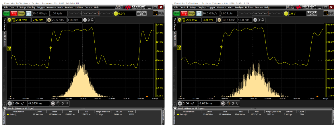
(a) Measurement of the clock output CLK_ADC2 close to the LMK04806, \sigma_{t,\text{period}} = 2.7\ \text{ps}_{\text{RMS}} . (b) Measurement of the clock output CLK_ADC2 close to the LTM9009-14, \sigma_{t,\text{period}} = 3.5\ \text{ps}_{\text{RMS}} .
