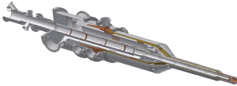
Figure 2.9.: The Bonn Frozen-Spin Target with part of the holding structure. The target cell with the holding coil is situated at the very front. [40]
