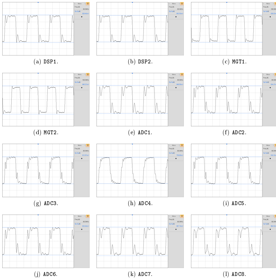
Figure D.1.: Waveforms of the clock signals, measured close to the PLL (LMK04806). DSP are the clocks for the DSP algorithms, MGT are the clocks for the network interface, ADC are the ADC digitization clocks (cf. Figure 5.8). All signals show artifacts, possibly from non-ideal matching of termination and trace impedance.
