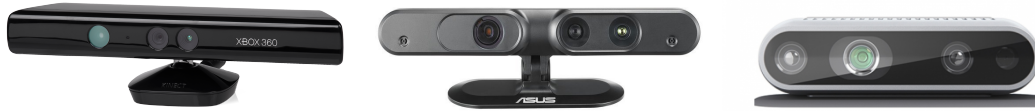
Figure 2.1: Example of RGB-D sensors. From left to right: Microsoft Kinect, Asus Xtion Pro Live, Intel RealSense D435. Courtesy of Microsoft, Asus and Intel.
