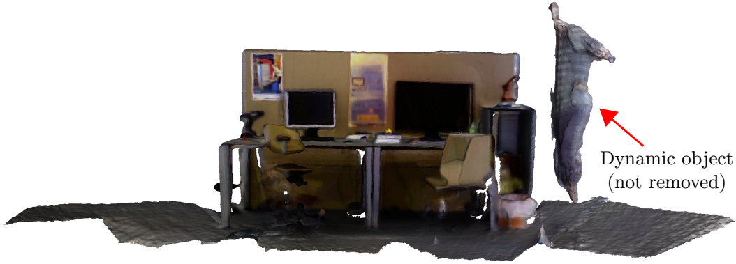
Figure 6.9: Final mesh obtained using our approach on the walking_xyz sequence. In this sequence, the camera follows the person on the right at the beginning and then never revisits that location. Therefore, the person is added in the model.
