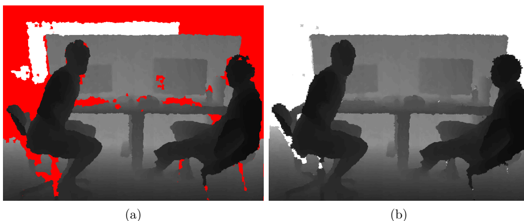
Figure 6.6: (a) Raw depth from the RGB-D sensor. Out-of-range values are highlighted in red. (b) Our virtual refined depth from 10 adjacent frames. (about 0.3s delay)
