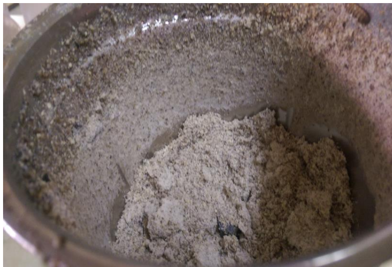
Figure 9.9 I used liquid nitrogen to dry the insect samples and a heavy-duty mixer/blender to crush them into powder prior to starting the nutritional analysis. Though the procedure was practical and handy, the liquid nitrogen was too costly, and I soon had to use oven heat instead.
