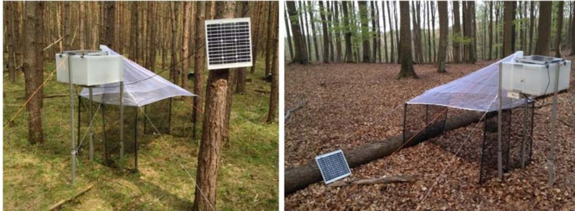
**Figure 5.6:** Typical pine (left) and beech plot (right) at the end of April with Malaise trap and automated interval sampler with installed solar panels (experimental plots SEW2 and SEW9; Struwe 2015).
