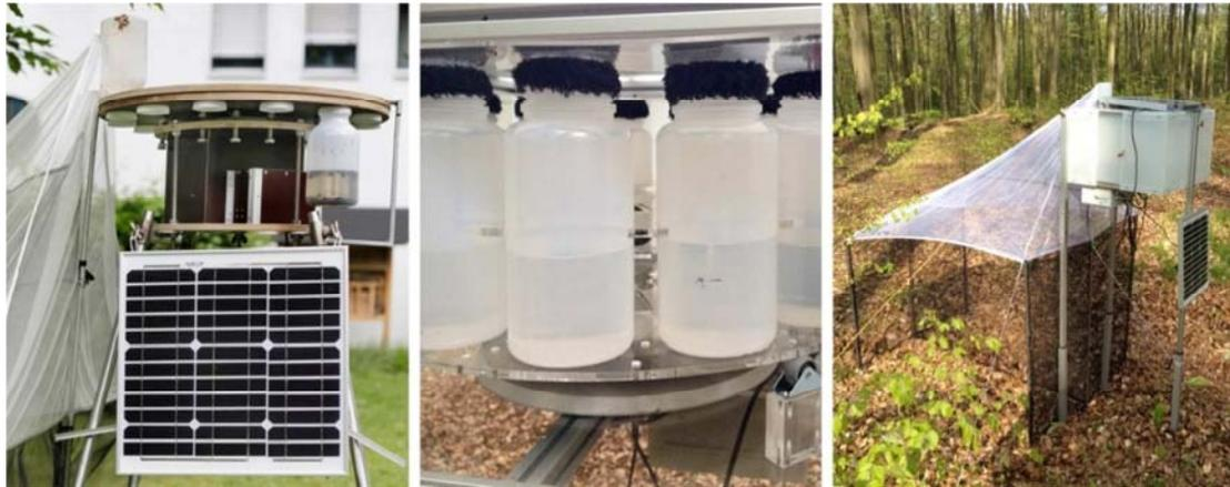
**Figure 5.1:** From left to right: (1) Prototype version of the automated interval sampler (AIS) with a single hanging storing-jar and solar panel. (2) Inside of the acrylic housing of the second version with storing jars with black sealing rings fixed upon on a rotating plate filled with ethanol. (3) AIS set up with Malaise trap in the Schorfheide-Chorin on plot SEW7 (Photos: Struwe 2015).
