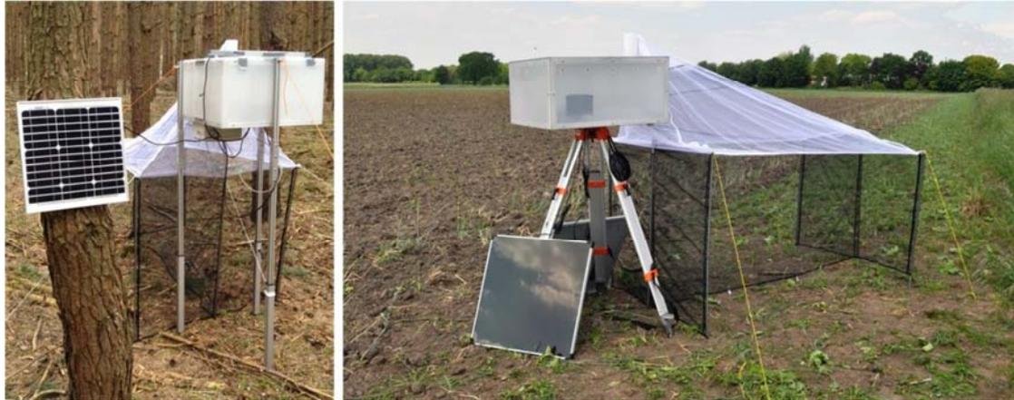
**Figure 5.13:** Left: The automated interval sampler (AIS) as it was used in the Schorfheide-Chorin together with a Malaise trap on plot SEW15 (Photo: Struwe 2015). Right: The current AIS version with improvements (Photo: Kilian 2017).
