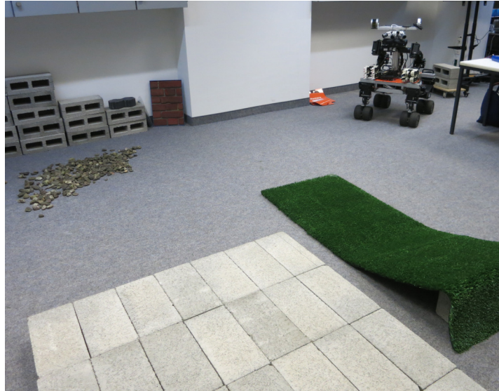
Figure 3.25: Scenario for the real robot experiment with Momaro including a field of gravel, a patch of grass, and an elevated platform. The shown robot state is its start state.
