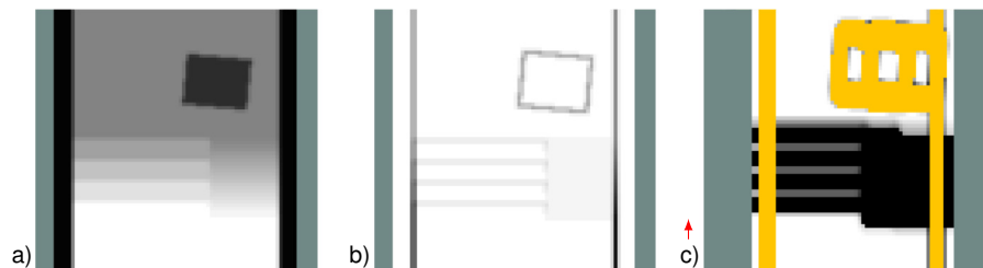
Figure 4.8: Level 2 environment representation. a) Height map. b) Height difference map. c) Foot pair cost map for the orientation indicated by the red arrow.
