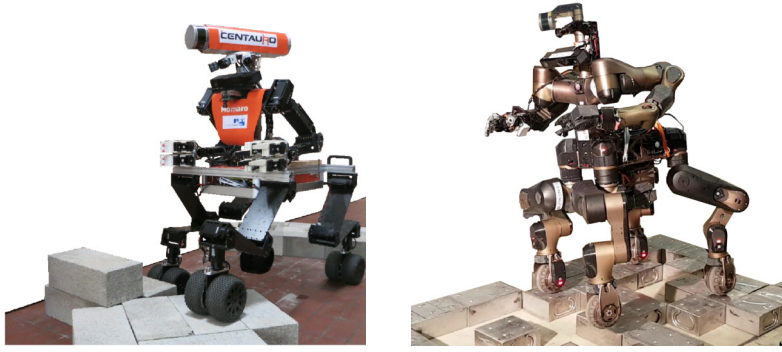
Figure 5.2: Hybrid driving-stepping locomotion robots addressed by the presented planning method. Left: Momaro. Right: Centauro
