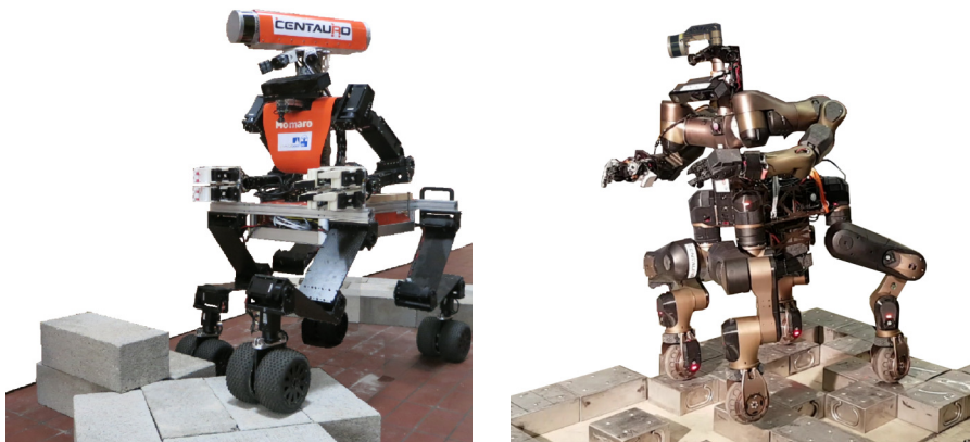
Figure 3.1: Hybrid driving-stepping robots employed with the described approach. Left: Momaro. Right: Centauro.
