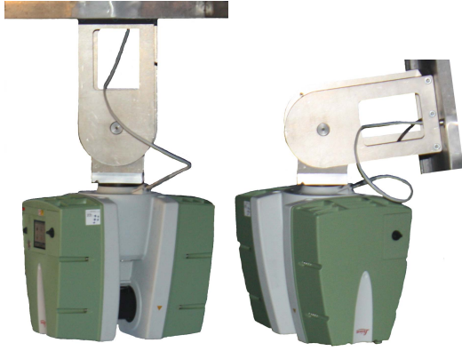
Fig. 3. Station and orientation of the TLS at an elevation angle of the telescope of 90 deg (left) and 7.5 deg (right).
