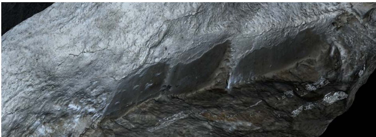
Figure 4. Detail of the upper left edge with parallel chainsaw marks and mortar deposits on the backside. Phong rendering with color texture.
