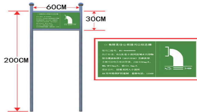
Figure 6.2 A standardized sign near the wastewater outfall of the enterprises
