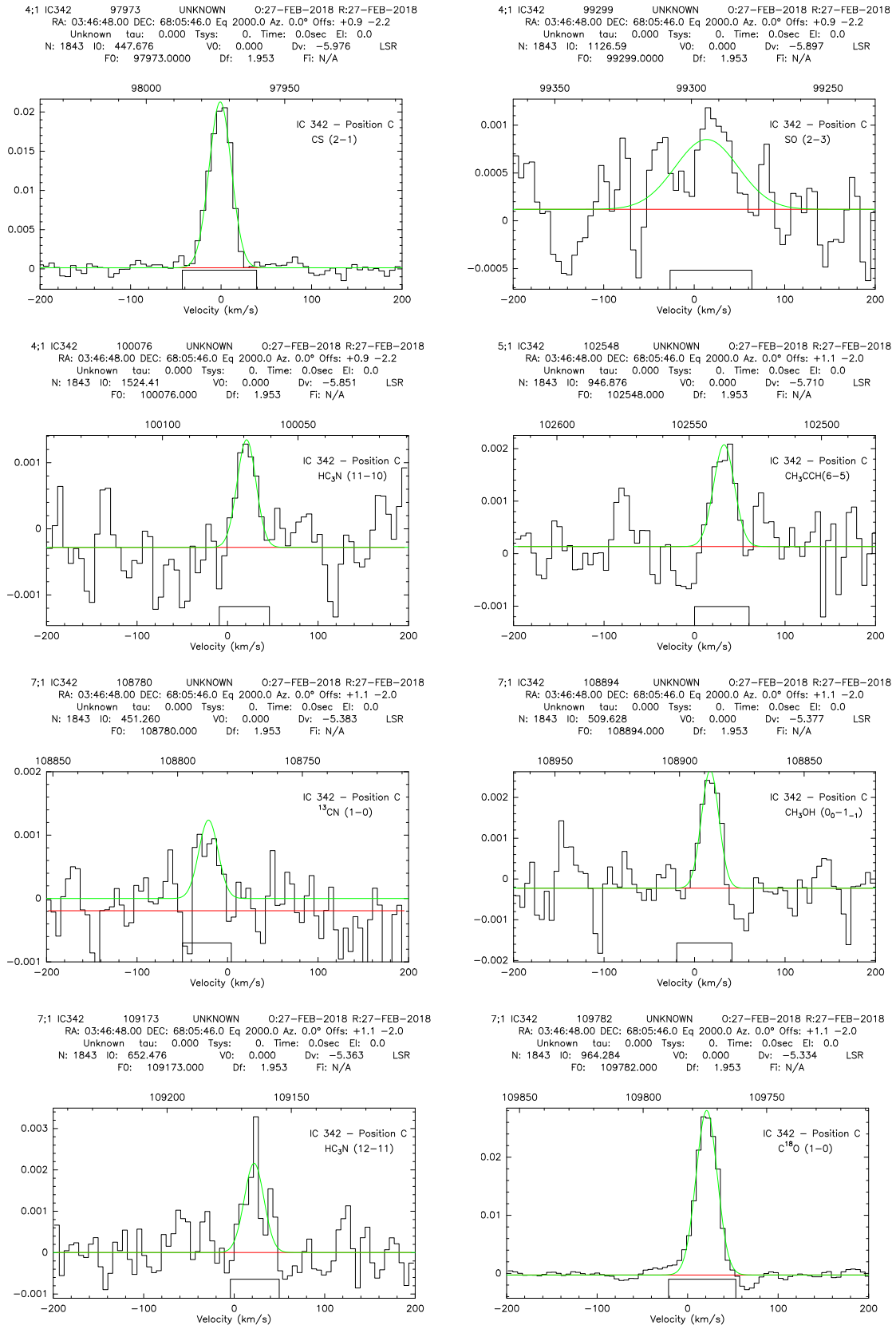
Figure D.23: IC 342: Spectra and Gaussian fit of CS(2 – 1) at 97.973 GHz, SO(2 – 3) at 99.299 GHz, HC 3 N(11 – 10) at 100.076 GHz, CH 3 CCH(6 k – 5 k ) at 102.548 GHz, 13 CN(11 – 10) at 108.780 GHz, CH 3 OH(0 0 – 1 -1 ) at 108.894 GHz, HC 3 N(12 – 11) at 109.173 GHz, and C 18 O(1 – 0) at 109.782 GHz. The axes are the same as in Fig. D.1.1
