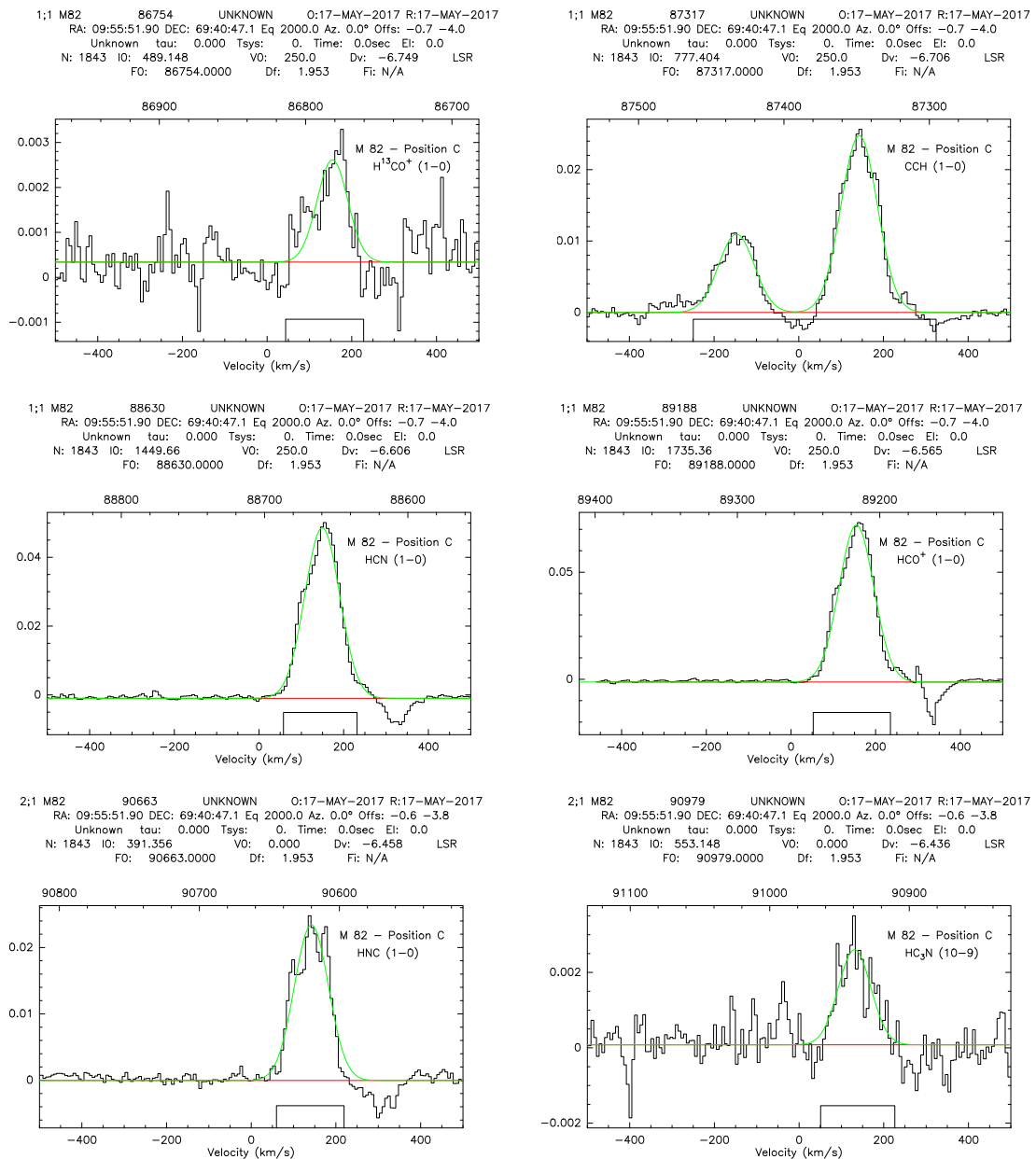
Figure D.7: M 82: Spectra and Gaussian fit of \text{H}^{13}\text{CO}^+(1-0) at 86.754 GHz, CCH(1-0) with 2 components at a central frequency of 87.317 GHz, HCN(1-0) at 88.630 GHz, \text{HCO}^+(1-0) at 89.188 GHz, HNC(1-0) at 90.663 GHz, and \text{HC}_3\text{N}(10-9) at 90.979 GHz. The axes are the same as in Fig. D.1.1
