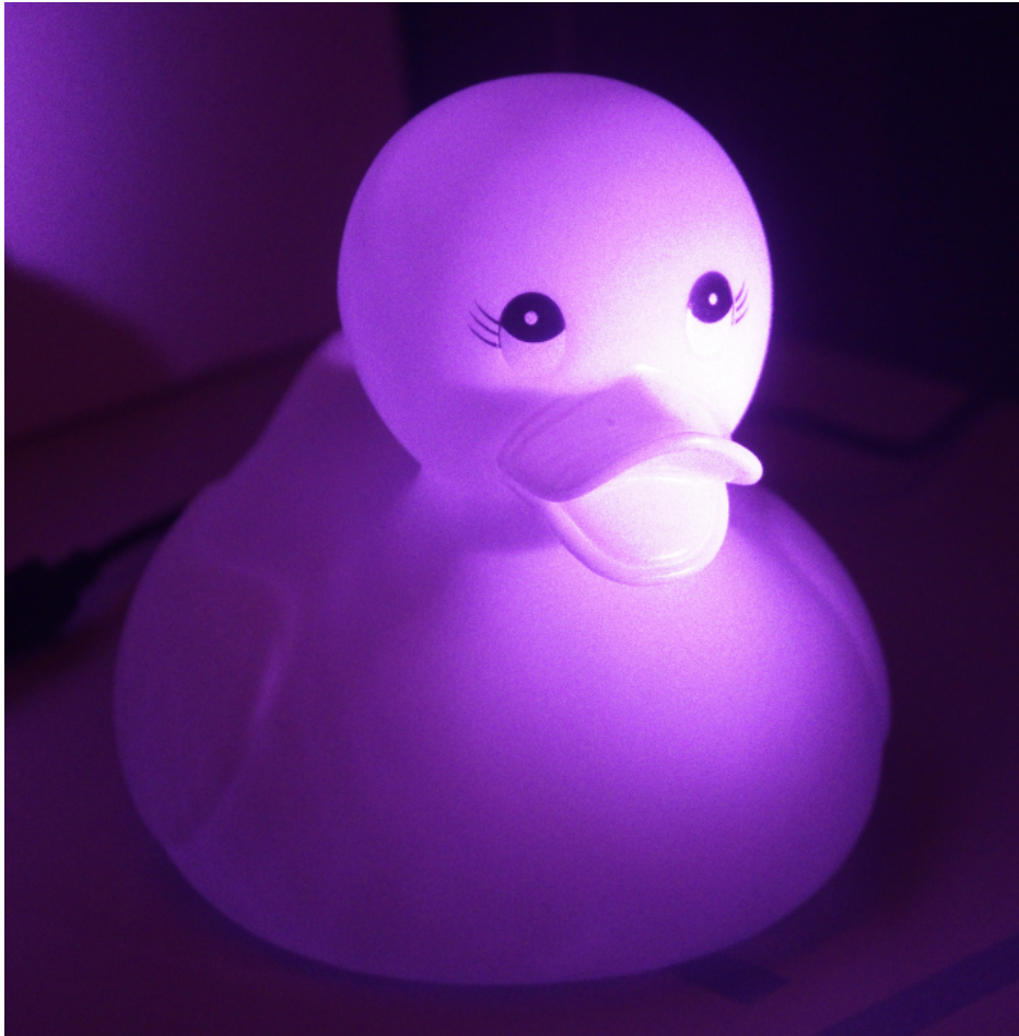
Figure 3.14: The rubber duck target we use to showcase measurements of a translucent material. The image was taken under infrared illumination at 852 nm using our laser light source in combination with an IR camera. Internal scattering within the material is visible, visualizing the complex light transport involved.
