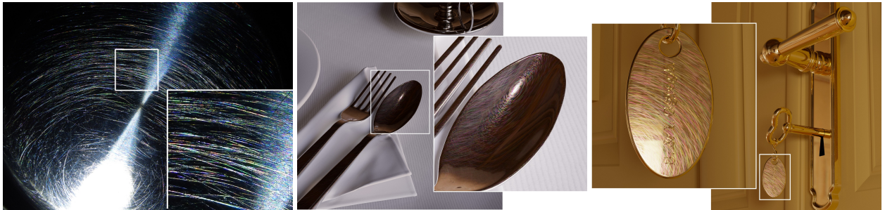
Figure 5.1: Left: Inside of a cooking pot photographed under a halogen spotlight. Center and right: Renderings of scratched materials under environment lighting obtained using our model.
