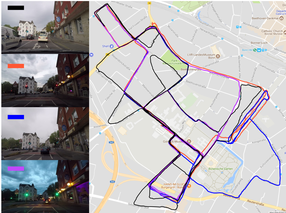
Figure 6.1: Example dataset, where the map consists of three trajectories collected in different points in time as well as in different weather conditions. The corresponding image sequences cover also partially different routes. The query trajectory depicted in black.
