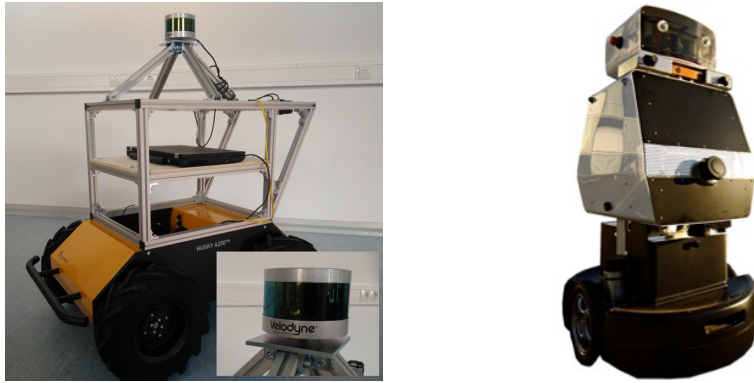
Figure 8.6: Robots used in our experiments: robot equipped with Velodyne VLP-16 laser scanner mounted parallel to the ground (left) and a Velodyne HDL-32E mounted on the head of the Obelix robot from the AIS lab of the University of Freiburg (right).
