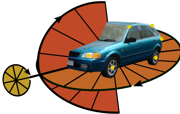
Figure 1.9: Visualisation of the 3 viewpoint angles, i.e. azimuth (orange), elevation (red) and tilt (yellow), and the keypoints of a car. The displacement of the non-occluded keypoints will remain the same for all car instances that are placed with the same pose.
