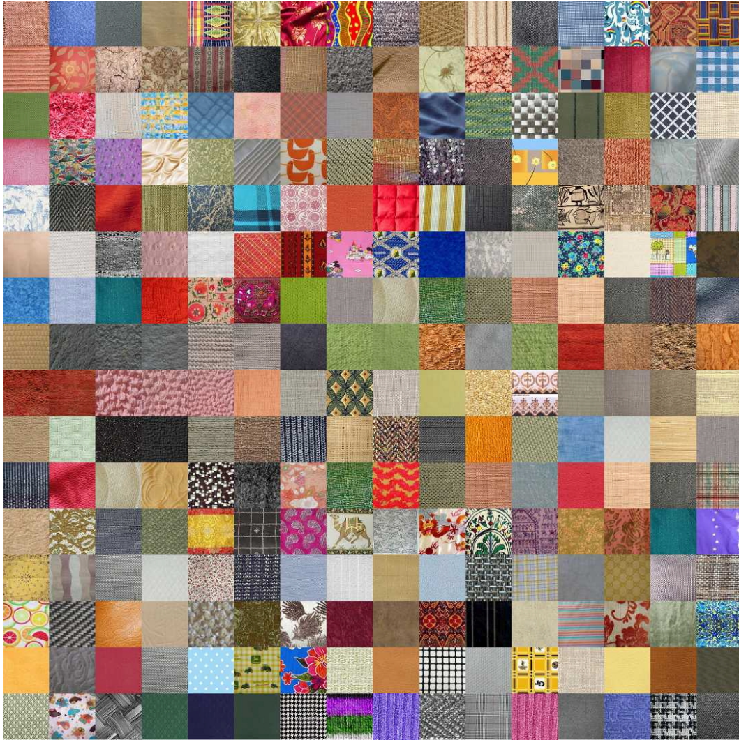
Figure 4.2: From [GZ13]: Material patches, used in Giesel and Zaidis affordance classification experiments. The researchers cropped 256 color images of fabrics to a size of 150 x 150 pixels. Images were presented on a monitor against a black background. The viewing distance was 70 cm.
