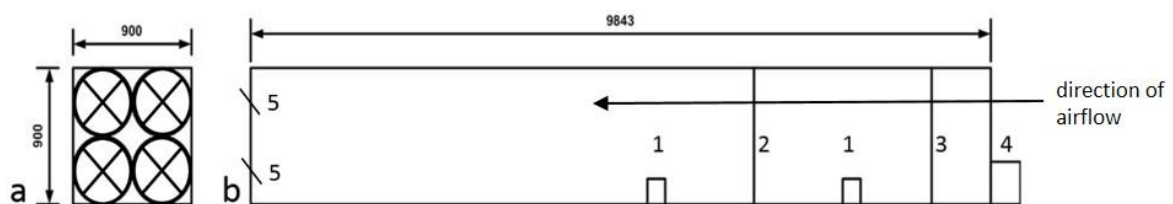
Figure 1: schematic draft of the wind tunnel. a: front view onto the four axial fans (Ø 300 mm each); b: side view onto the wind tunnel, 1: position of the aerosol spectrometers, 2: filter wall, 3: flow straightener, 4: position of the dust inlet, 5: position of the fans. Dimensions in mm
