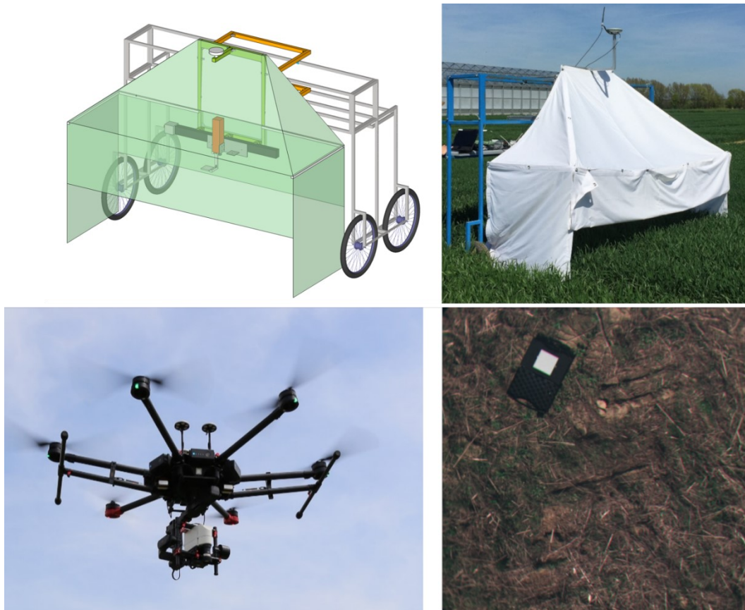
Figure 3. Construction plan of the Phytobike (top left) and the final appearance in the field including the cotton diffusor (top right). The used UAV system consisting of a DJI Matrice 600 and a Rikola hyperspectral camera (bottom left). Normalization was performed using a 50 % grey reference panel (bottom right).
