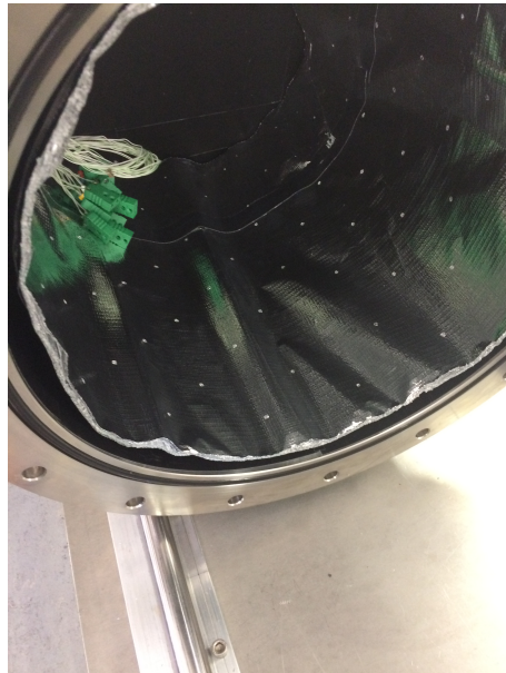
Figure D.4: Optional MLI foil inside the vacuum vessel.
