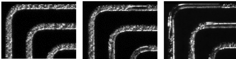
Figure 9.3: Flow boiling of CO 2 in multi-micro-channels recorded at Position 2, T_{sat} variation left to right: 15°C, 5°C, -25°C.
