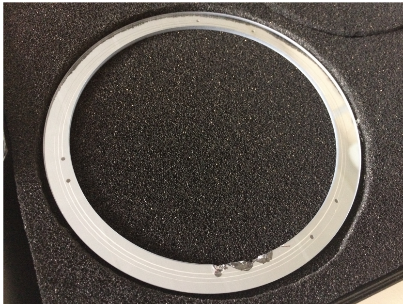
Figure C.5: Failure of the water jet dicing method II.
