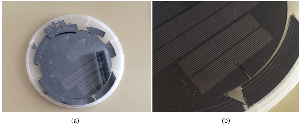
Figure C.3: Failure of the water jet dicing method I: a) damaged outer annulus ; b) damaged inner part.
