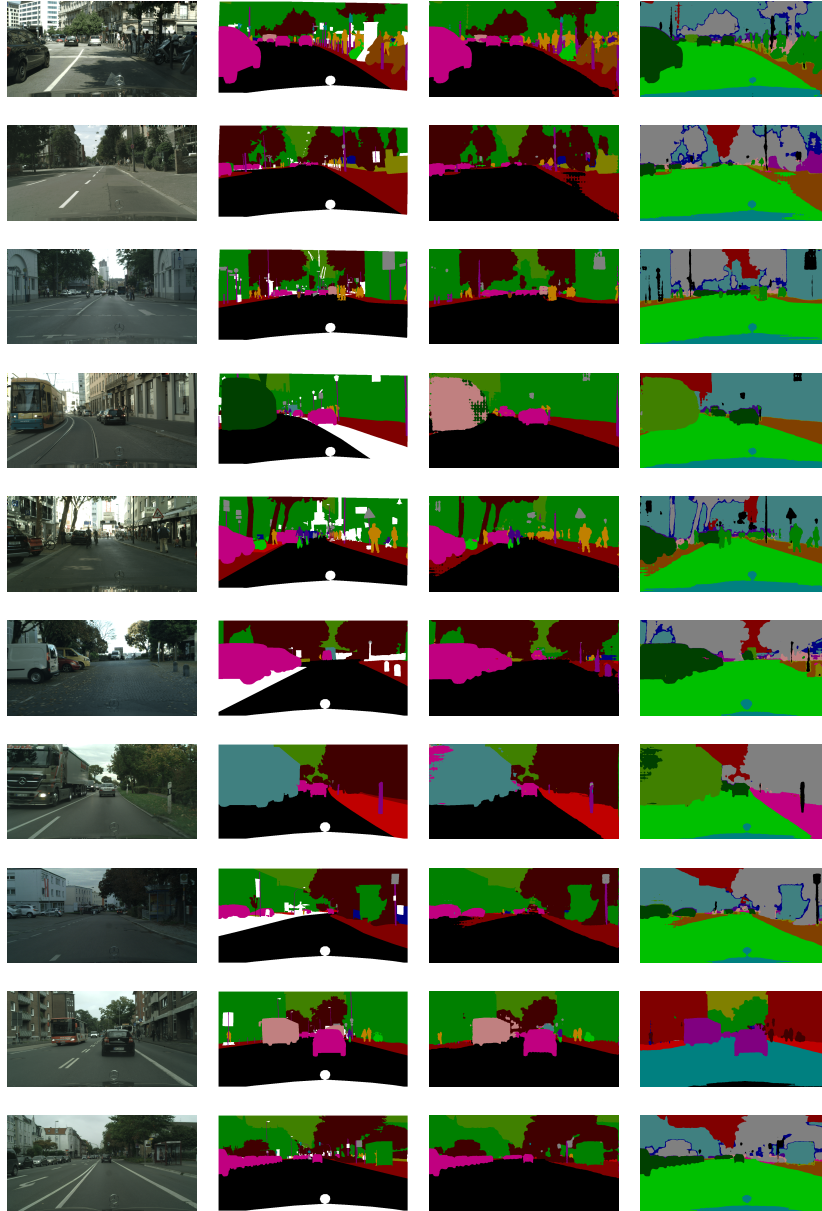
Figure 8.4: Qualitative examples from the Cityscapes val set. From left to right: image, ground truth, proposed, latent classes.
