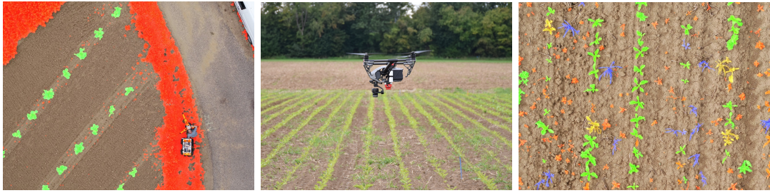
Figure 4.16: From left to right: analyzed image by our approach classifying pumpkin (green) and weed (red). UAV operation in a sugar beet field. Multi-class prediction of an image of a sugar beet field considering sugar beet (green), weed (red), grass (blue) and mixed (orange).
