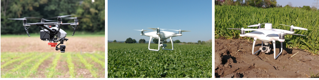
Figure 3.6: Different UAVs used for data acquisition. Left: DJI Phantom 4 with built-in RGB camera. Middle: DJI Inspire II with DJI Zenmuse X5s RGB camera. Right: DJI Phantom 4 RTK with built-in RGB camera
