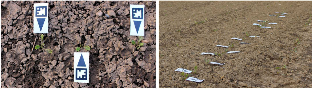
Figure 4.15: Labeling of the crop plants (sugar beets) with markers placed next to the plant. We find the markers in the images and assign the label “crop” to detected vegetation based on a distance threshold, all other vegetation is considered to belong to the “weed” class.
