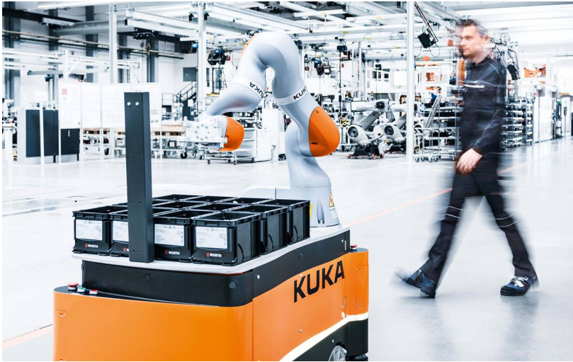
Figure 4.1: A KUKA KMR iiwa mobile manipulator deployed on a factory floor where it shares the workspace with human operators as in the use case envisioned by the RobDREAM project. Image courtesy of KUKA Roboter AG.
