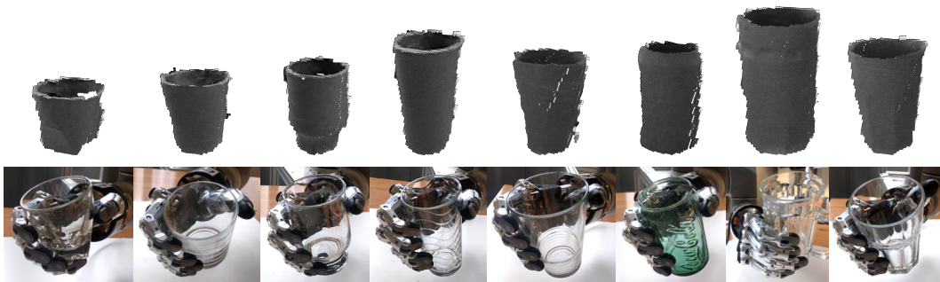
Figure 5.7: Training Glass instances for the synergy learner. Top: observed point clouds, and bottom: the corresponding grasps performed through teleoperation with the exoskeleton.
