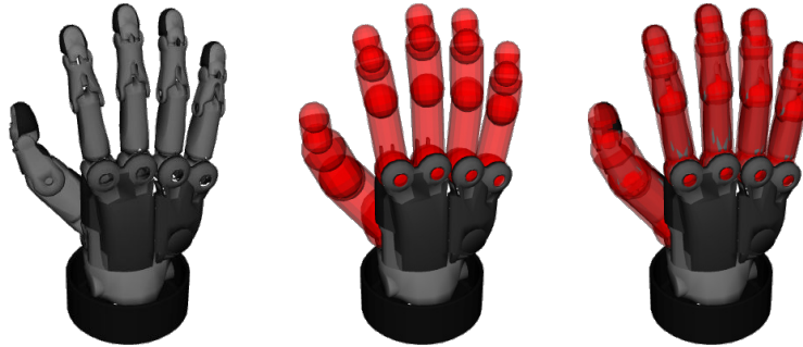
Figure 4.8: Collision model of the Schunk SVH hand approximated by geometrical primitives. Left: Detailed 3D model of the robotic hand. Center: fingers modeled as capsules. Right: visual and collision model of the robotic hand to show the quality of the capsule approximation.
