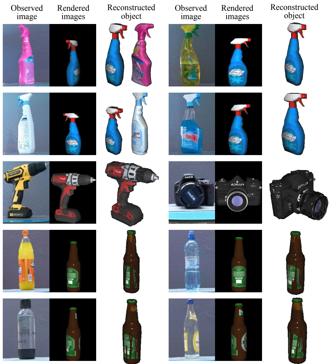
Figure 3.11: Results of the non-rigid registration on real RGB images. When available, the 3D ground truth object models are displayed next to the deformed instances. Our method is able to successfully register objects with transparent surfaces which are normally hard to perceive by 3D sensors.
