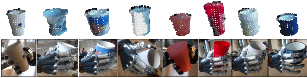
Figure 5.10: Synergy learner evaluation on real glasses. All the instances are novel to our approach and are successfully grasped.
