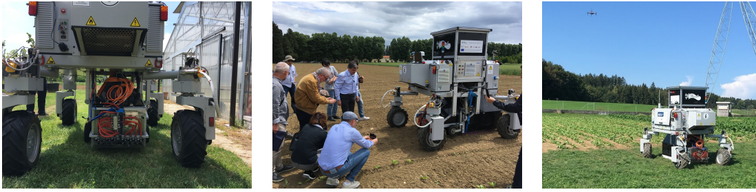
Figure 6.1: Photos from various integration and review meetings of the Flourish project. Left: Integration of the precision spraying system on the robot for weed treatment. Middle: Demonstration of precision weeding capability in autonomous mode to local farmers and other stakeholders in Ancona, Italy. Right: The UAV and UGV team entering the field for final project demonstration in Eschikon, Switzerland.
