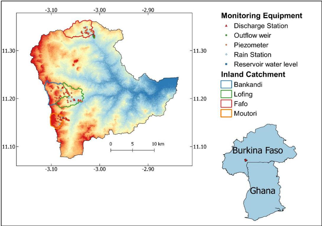
Figure 3.1: Dano basin and selected catchments with monitoring equipment
