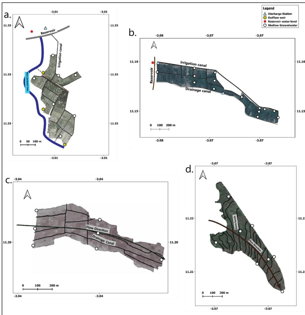
Figure 3.2: Selected schemes with: (a) Reservoir with irrigated schemes in Fafo, (b) Drainage canals in Lofing, (c) Reservoir with irrigated scheme in Moutori, and (d) Contour bunds in Bankandi
