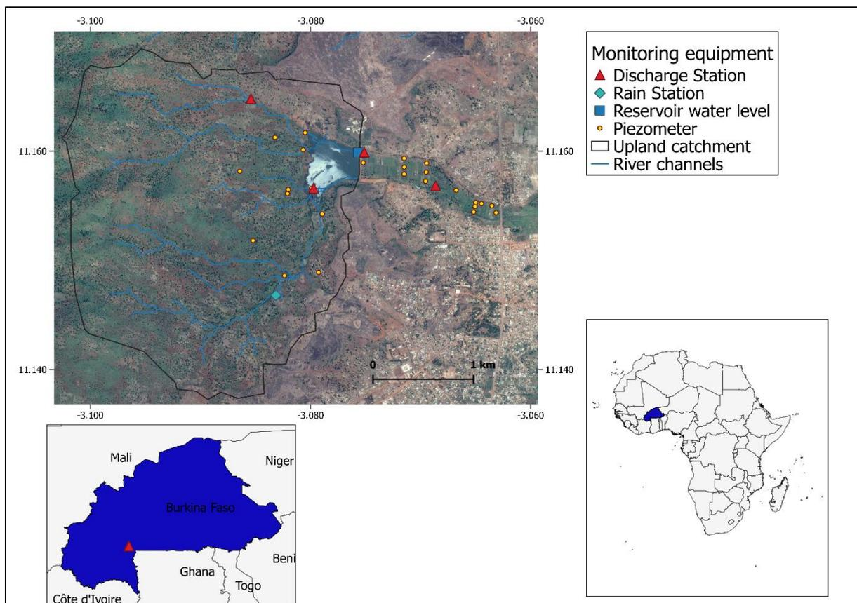
Figure 2.1: Equipment and monitoring locations in the reservoir-based scheme in Moutori.
