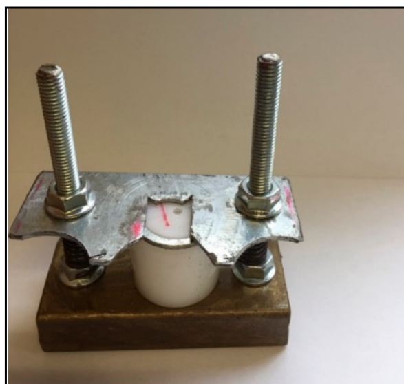
Figure 4. Teflon mold fixed by a metallic device with screws on the tooth surface for bond strength specimen preparation.
