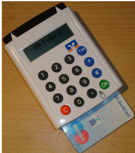
Figure 8.4: A SmartTAN Optic TAN generator from a German bank. The customer's card is inserted into the device, transaction data is transmitted through optical sensors by holding the token in front of a flickering code on screen. As a fallback mechanism, the data can also be entered through the device's keypad. After the relevant transaction data is displayed on the screen and acknowledged by the user, the device eventually displays the TAN.
