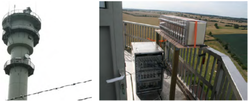
Figure 8.1: Receiver system GAMMA-2. (a) GAMMA-2 mounted on the tower; (b) GSM PCL antenna and GAMMA-2 receiver
