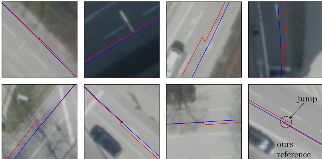
Figure 6.5: The figure shows cases in which the reference trajectory is inaccurate and unusable for our evaluation. This is based on sudden changes, i.e., jumps, in the reference trajectory as, e.g., shown in the bottom right image. Whenever there is a jump in the reference trajectory, the reference system corrects previously accumulated drift. Consequently, the preceding segment of the reference system is inaccurate and thus unusable for our evaluation. We manually identified these problematic segments and excluded the corresponding parts from our evaluation. The trajectory estimates of our system are only shown for visual comparison. Aerial images by Landesbetrieb Geoinformation und Vermessung (2019).
