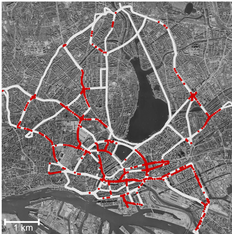
Figure 6.18: GNSS outages over 10 s. The parts of the trajectories for which the low-cost GNSS receiver could compute a pose estimate within ten seconds are shown in white. Vice versa, the locations in our dataset for which the low-cost GNSS receiver was not able to compute a pose estimate for over ten seconds are shown in red. These outages mainly occur in areas with blocked line-of-sight like tunnels, bridges, and urban canyons. Overall, roughly 18% of the overall recorded trajectories are within a GNSS outage phase. Aerial images by Landesbetrieb Geoinformation und Vermessung (2019).
