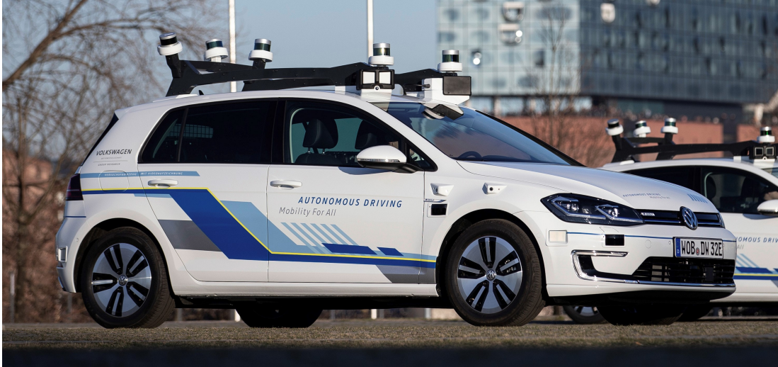
Figure 6.3: The prototype e-Golf used in our experiments. It is equipped with various sensors, as illustrated in Figure 6.4. Source: Volkswagen AG (2019).
