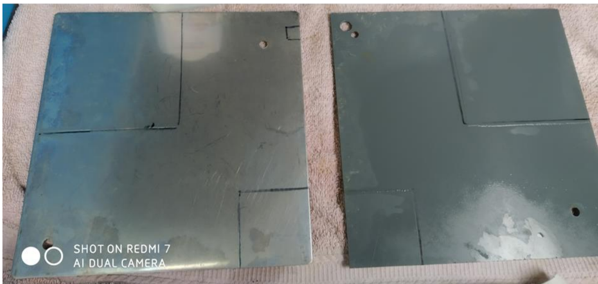
Figure 49: Plates after removal from Cooling Tower 4.
