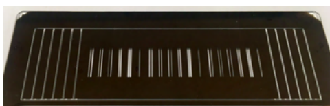
Figure 3.5: Quartz photo-mask for fabrication of 3D hydrogel structures. The photomask holds pairs of rectangular structures that frame the gradient area of the chemotaxis chambers when a \mu -Slide Chemotaxis is placed on the mask and aligned. The slide dimensions (25x75 mm) are outlined on the mask to help achieve a precise alignment. The photomask enables fabrication of structures of varying width and spacing (0.3–0.5 mm/0.1–0.6 mm), resulting in migration arenas of various size. For the chemotaxis assay, the 300 \mu\text{m} wide structures proved to be most suitable, enclosing a 400 \mu\text{m} wide arena between the hydrogel barriers.
