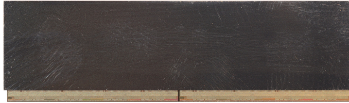
Figure 8.4: A bare RD53A DCM (Combination C6). The metallization on the sensor backside (top) appears dark. The metallization layer is scratched due to an invasive metrology measurement. The bottom part of the two RD53A readout chips with the wire-bond pads can be seen at the bottom.
