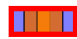
(e) Minimum area violation. All metal components must have at least some given area.
