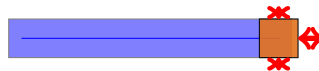
(g) Via extension errors. The metal on a routing layer needs to extend a certain distance over the projection of the middle shape in each direction.
