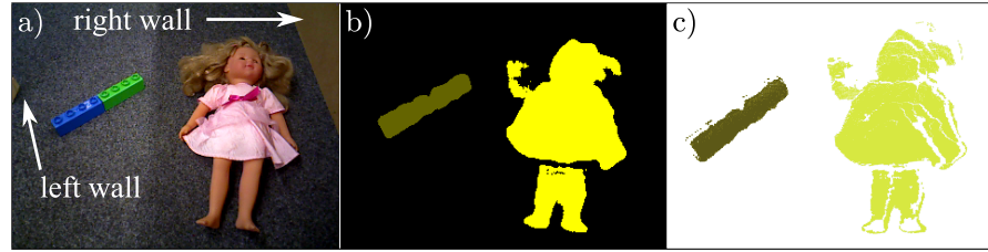
Figure 7.11: Data processing for the RGB-D data. a) The original RGB image containing a doll and toy blocks between two walls. b) Semantic segmentation results using the Bonnet framework. c) Segmented point cloud of the corresponding objects, using the depth image to get the spatial information of each marked pixel.
