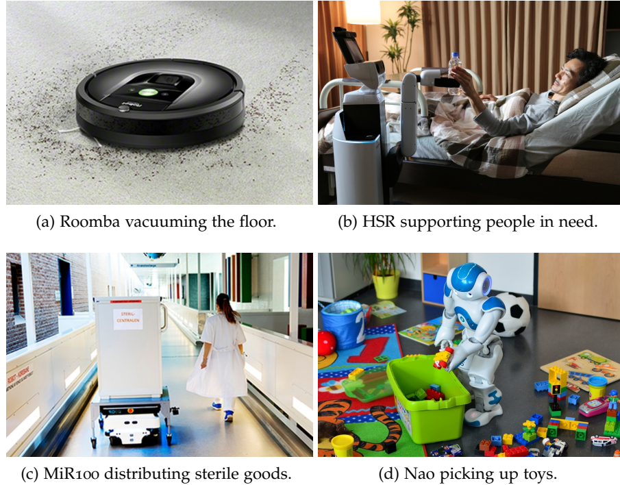
Figure 1.1: Robots operating in human environments. a) The iRobot Roomba vacuum cleaner is widely used in many households (source: [6]). b) Human Support Robot (HSR) designed by Toyota for collaborative task in a household environment (source: [7]). c) The MiR100 model developed by Mobile Industrial Robots is already deployed in a hospital for automated logistic tasks (source: [2]). d) The educational and research robot NAO from SoftBank Robotics is also used for entertainment and information purposes (source: [8]).
