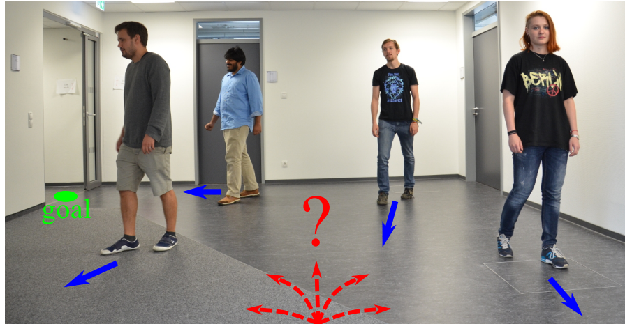
Figure 5.1: Example of a robot navigating through environment populated by humans. To avoid collisions and efficiently reach the goal, the robot has to decide on its control commands. We propose to use a neural network in combination with the popular social force model (SFM) to generate acceleration commands, based on features describing the configuration of the humans in the robot's vicinity.
