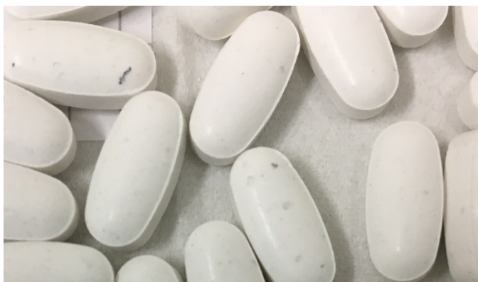
Figure 62 Tablets with visual defects caused by abrasion effects during twin screw wet granulation process
