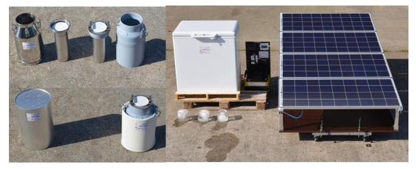
The strategy of milk cooling can be divided into two steps: the production of ice blocks through the use of a smart solar freezer in combination with a control panel that manages the solar energy to efficiently produce ice every day, and the cooling of milk done in the insulated milk cans as shown in Figure 2. The ice blocks produced are placed inside the ice compartment and when the insulated milk can is filled with milk, the ice compartment is placed inside the milk can.
