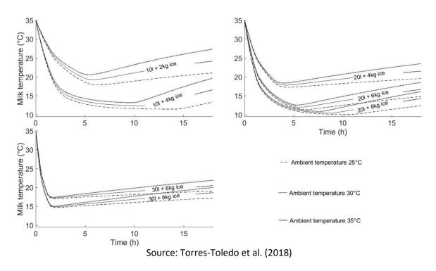
Figure 8: Cooling curves of different milk and ice ratios at different ambient conditions
