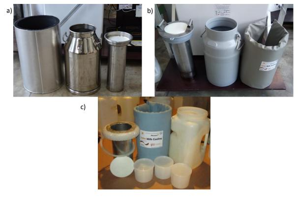
The cooling characteristics of the milk cans shown in Figure 6 were assessed under extreme ambient temperature of 35°C. It was evident that the stainless steel milk can requires a stronger insulation material, compared to the plastic milk can. Nevertheless, the plastic milk cans still required the insulation material in order to reduce the influence of ambient conditions in the cooling process of milk.
