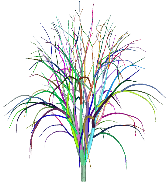
Figure 4.4: Exemplary segment hierarchy obtained from an initially provided plant segmentation: The artificially generated tree has a natural segmentation. We impose a hierarchy by heuristically or manually selecting a root (the tree trunk) and then performing successive nearest neighbor searches in order to generate a hierarchy on the segments.
