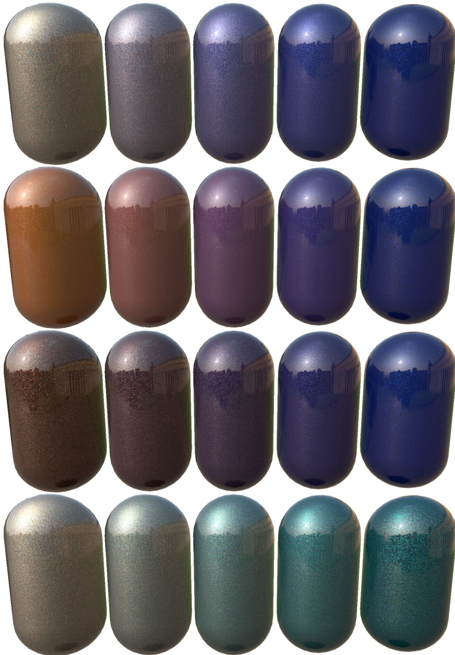
Figure 3.6: Several interpolations: In each row, the capsules in the left and right column are have been assigned the original measured paints, capsules have been assigned materials interpolated between the respective measured materials. The green-blue paint in the bottom picture is a flip-flop paint, which is also correctly interpolated. The flip-flop effect gets weaker the more one goes towards the gray paint.
