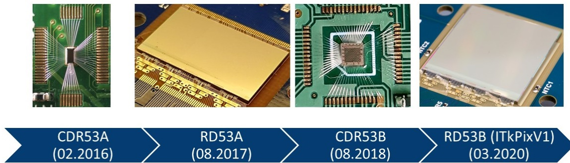
Figure 4.4: Photos of CDR prototypes and RD53 chips. The devices are arranged in the chronological order with the submission date indicated at the bottom. Chip sizes are very different: 2\ (4)\ \mu\text{m}^2 for CDR53A (CDR53B) and 2\ (4)\ \text{cm}^2 for RD53A (RD53B).
